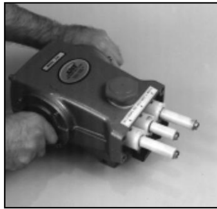
Proper Alignment of Ceramic Plungers for reassembly
