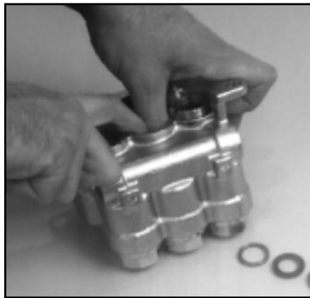
Installation of Male Adapter
